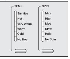
Press the "TEMP" and "SPIN" button until the indicator of the desired setting lights.
